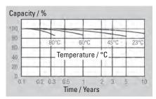
Self-discharge-rate referring to the ambient temperature
