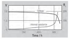
Typical discharge curve: Renata CR2540N at  $3.3k\Omega$
