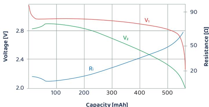
Figure: Pulse-current discharge characteristics<sup>1</sup> of the CR2450N cell. CR2450N Pulse intensity 10 mA, pulse width 50 ms, period 1 s. Cut-off voltage: 2.0 V
