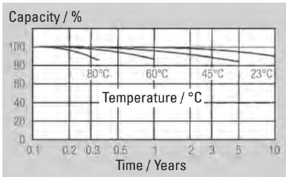
Self-discharge-rate referring to the ambient temperature
